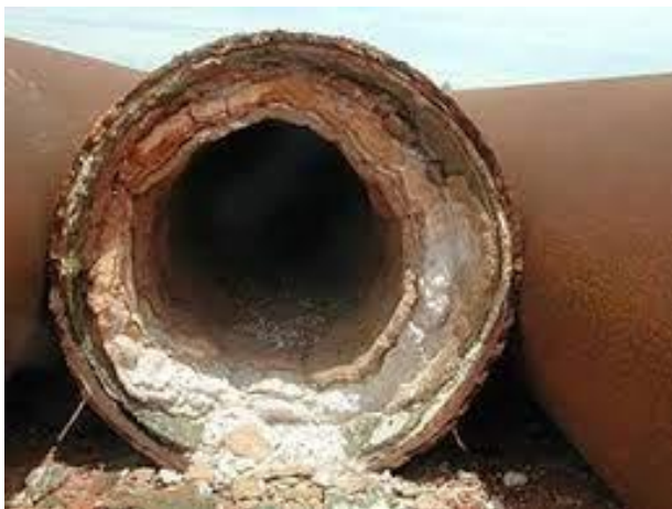
FIGURE 5 LIMESCALE BUILT-UP IN PIPES (ENVIROFLUID)
