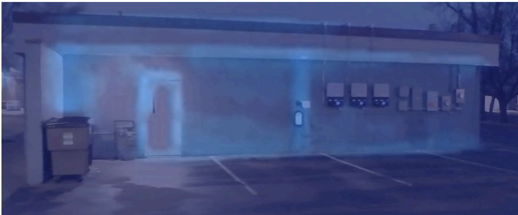
Figure 4: A thermal image taken by the drone of the right wall of the Morris City Hall The thermal image shows lower temperatures in darker blues and higher temperatures in lighter blues. The outline of the door on the left and the outline of the room partitions and ceiling are in light blue. The solar inverters are visible on the right side of the wall.
