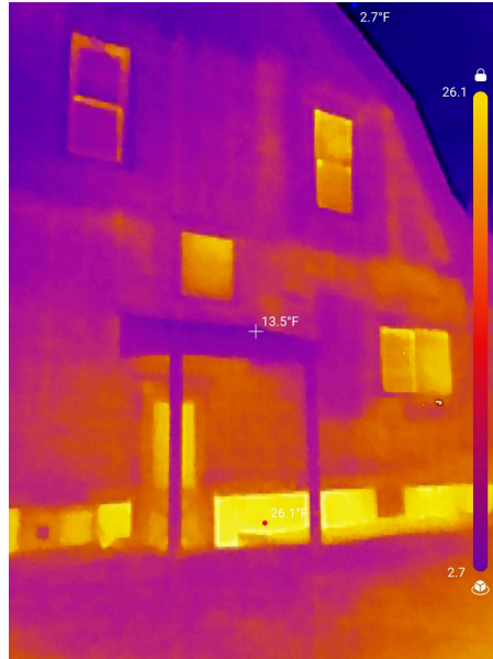
Figure 11. A thermal image of the side of Resident #3's home The temperature scale on the right of the image shows the lowest temperature as 2.7 Fahrenheit (purple) and the highest temperature as 26.1 Fahrenheit (yellow). The upper left window is purple-pink color while the other three windows are shades of yellow. The upper left window is not original to the house.
